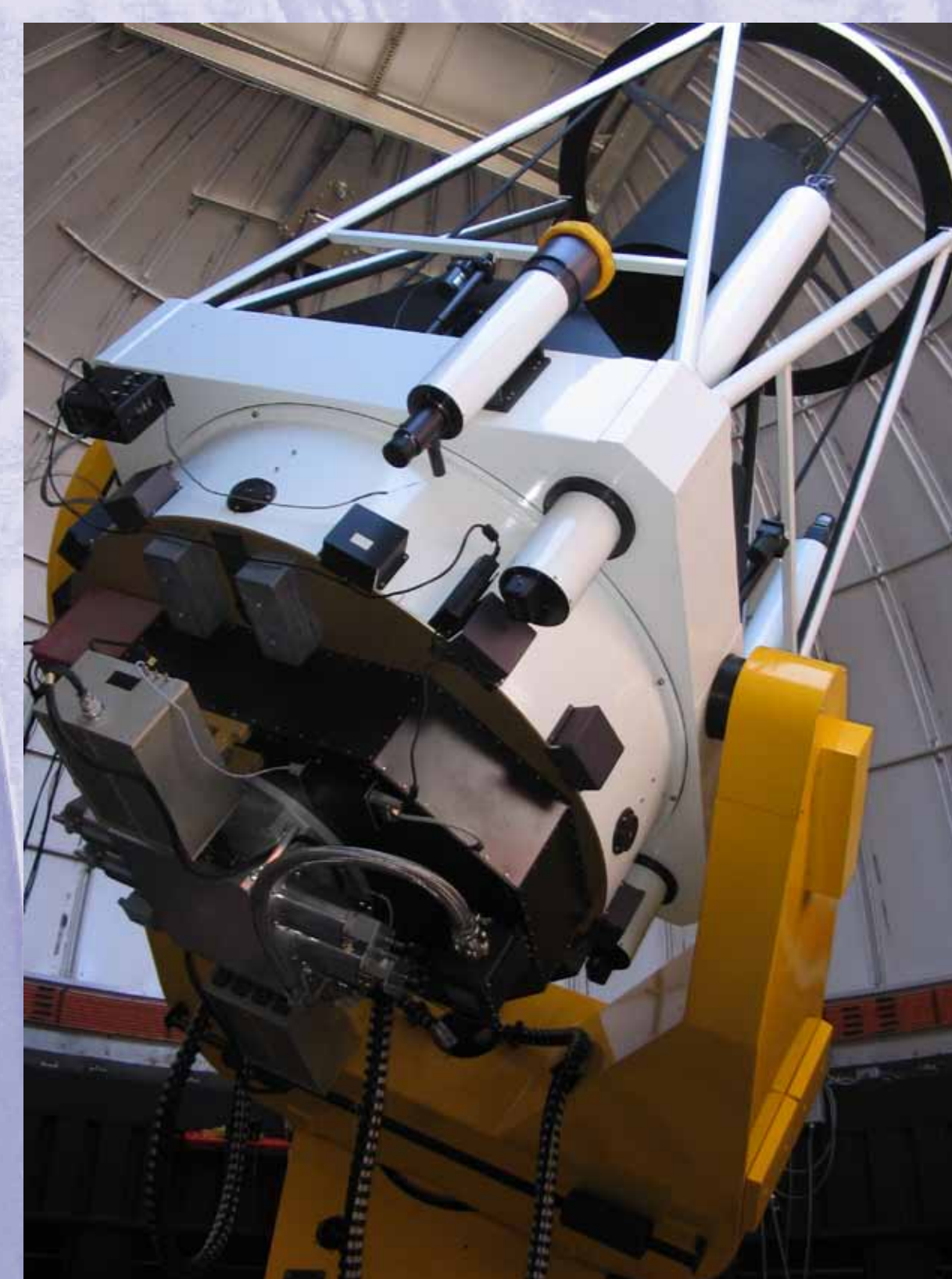
Polish telescope in Las Campanas in Chile. The Warsaw Telescope has a diameter of only 1.3 m, but its quality, equipment (above all the camera) and the manner of operation allowed for world-class discoveries, 2012
