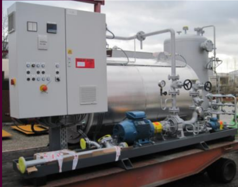
The boiler thermal oil heater - heat source of the ORC
