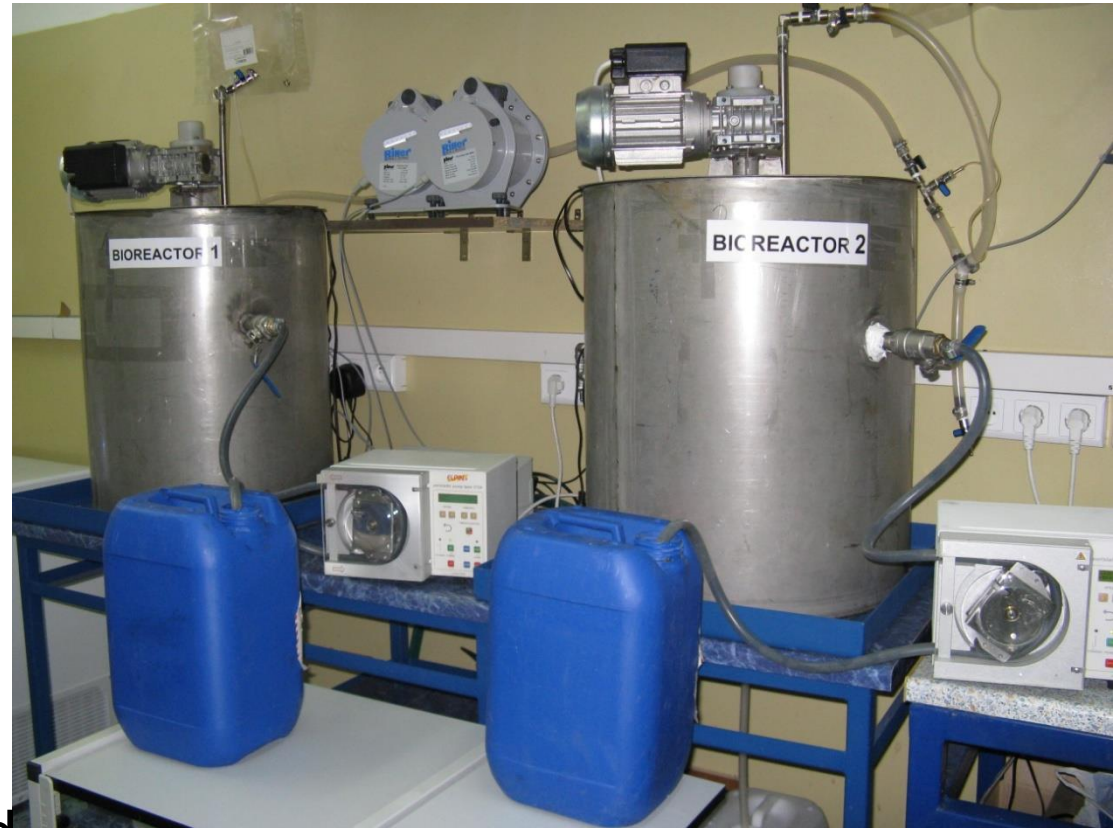
Part of the experimental set up for examination of biogas production from waste
