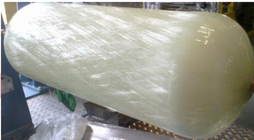
Manufacturing by winding technology
