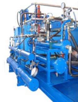
Hydraulic testing (according to ECE R110)
