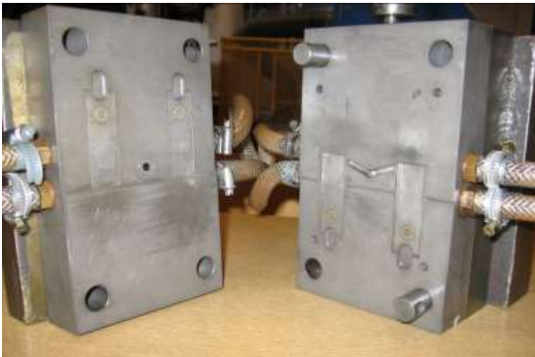
Injection mold for the investigations of bonding between metal and polymer
