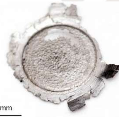
Sample processed by quasi-constrained high-pressure torsion
