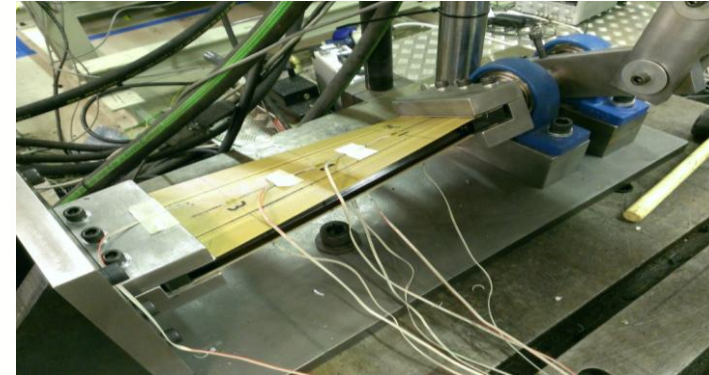
Testing of welded stiffened panel at Element Hitchin
