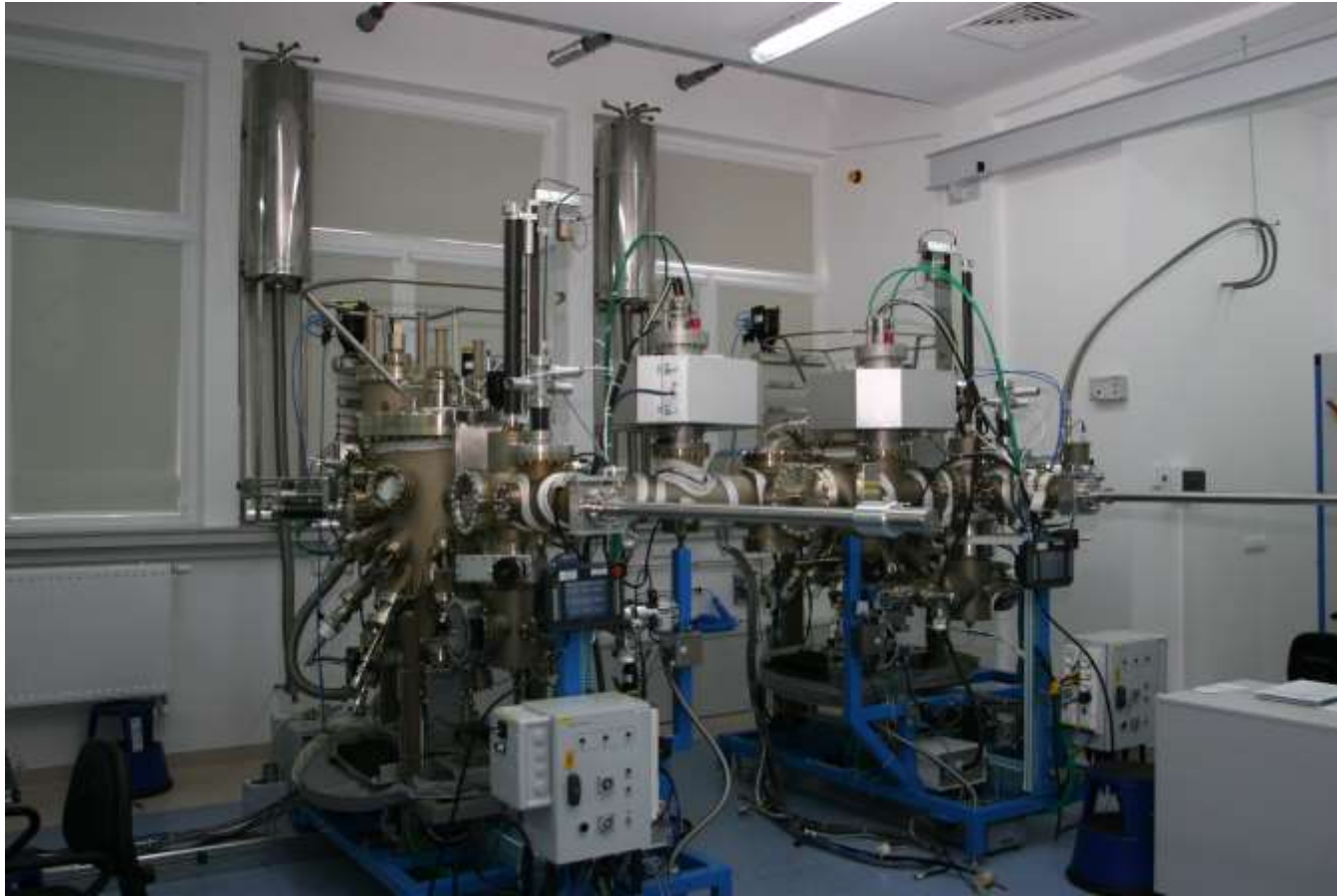
Double reactor MBE machine for the growth of ZnO and GaN heterostructures
