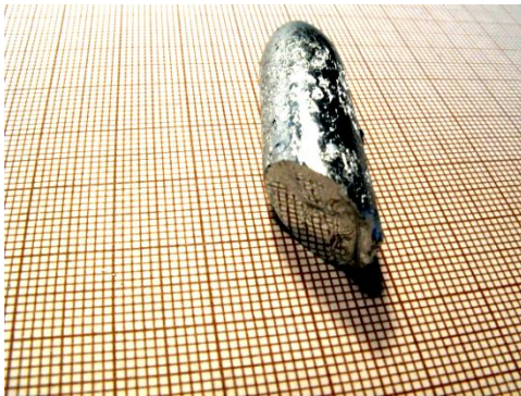
PbMnTe:Na bulk crystal ingot with Mn content x=0.01 grown by the Bridgman method (about half of the total length of a typical ingot shown).
